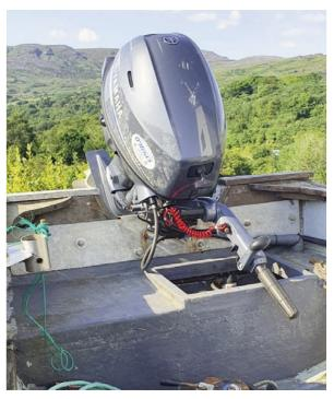
Photograph No. 5 - Inside the Boat with New Engine and Steel Bracket Fitted and Open Aft Locker.
