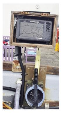
Photograph No. 6 - Sounder/Plotter and Hand Bilge Pump Fitted.
