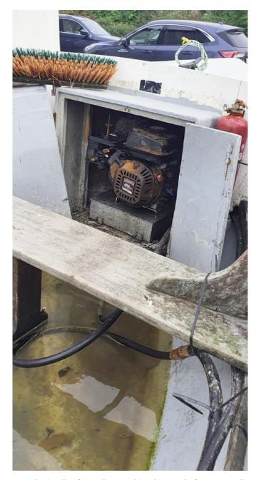
Photograph No. 7 - Open Forward Locker with Generator Fitted.
