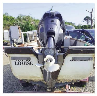
Photograph No. 3 - Stern View with Larger Engine (note the flat bars with bolts securing new bracket).
